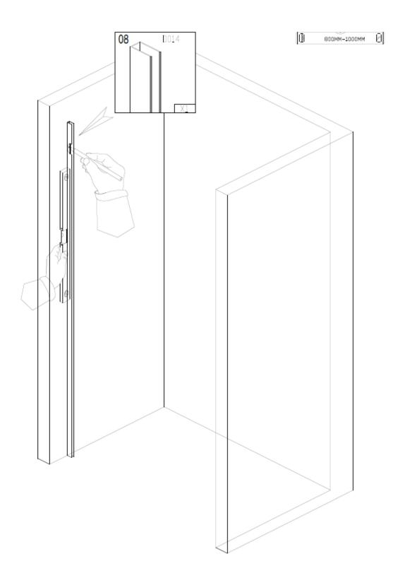
2. Place the aluminium profile against the wall, using a spirit level and a pencil to mark where holes will be drilled.
