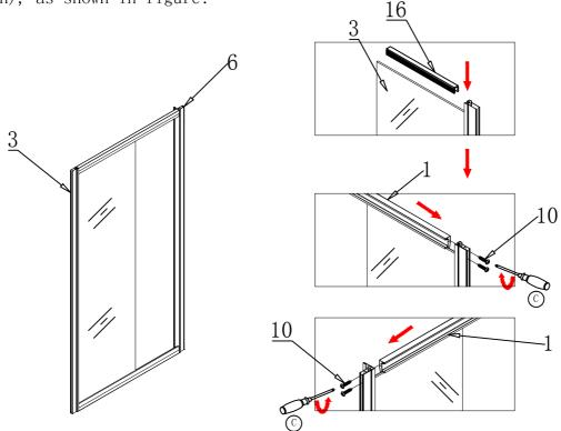
Step2:put the glass block to fixed glass, and then use a drill hole on the guide rail and tightening with self-drilling screw, as shown in figure:
