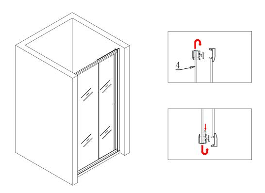
Step8: installed the weather bar and magnetic stripe as shown in figure (short weather bar loaded on the fixed glass, magnetic stripe note it's anode and cathode)
