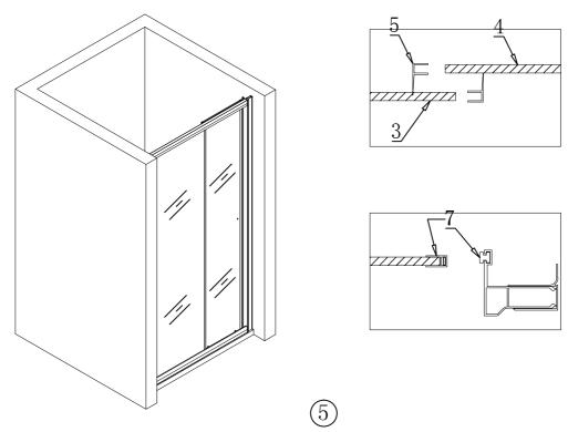
Step9: Install the door handle first, then use the cross screwdriver to adjust the pulley to make the difference in the activity gate consistent.
