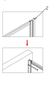
Step4: hole on wall and knock into the rubber plug, as shown in figure:
