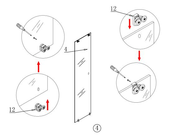
Step7: put the activity glass on the guide rail, as shown in figure:
