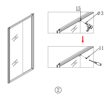
Step3: put the against the wall aluminum to the glass door, moved to the installation position and mark on the wall and open hole, as shown in figure.
