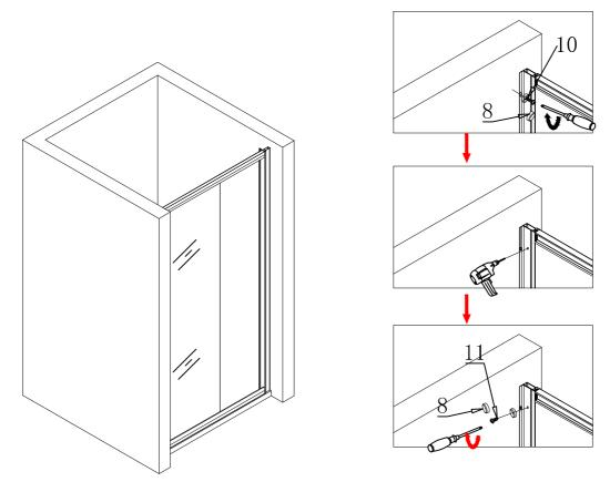
Step6: put the pulley to the active door, as shown in figure:
