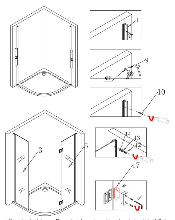
Place the aluminium profiles against the walls, marking where holes will be drilled.
