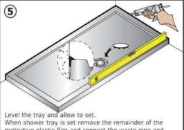
protective plastic film and connect the waste pipe and check for leakage.
