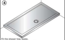
Ensure the two side edges are flat to the wall. Place the shower tray onto the cement bed and apply gentle pressure with the palm of the hand to bed the tray into position.
