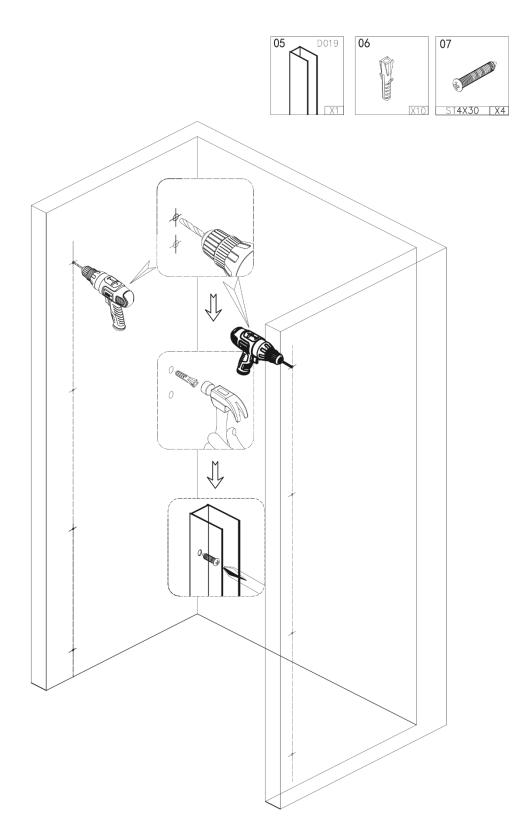
3. Drill the holes, inserting wall plugs and screwing the aluminium profiles onto each wall.
