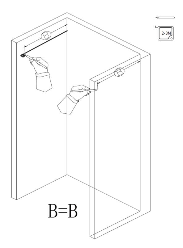
2. Place the aluminium profiles against the walls, using a spirit level and marking where holes will be drilled.
