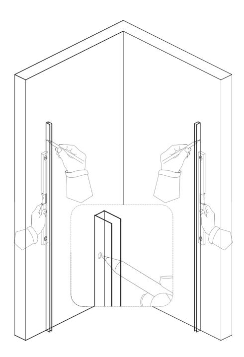
2. Place the aluminium profiles against the walls, marking where holes will be drilled.
