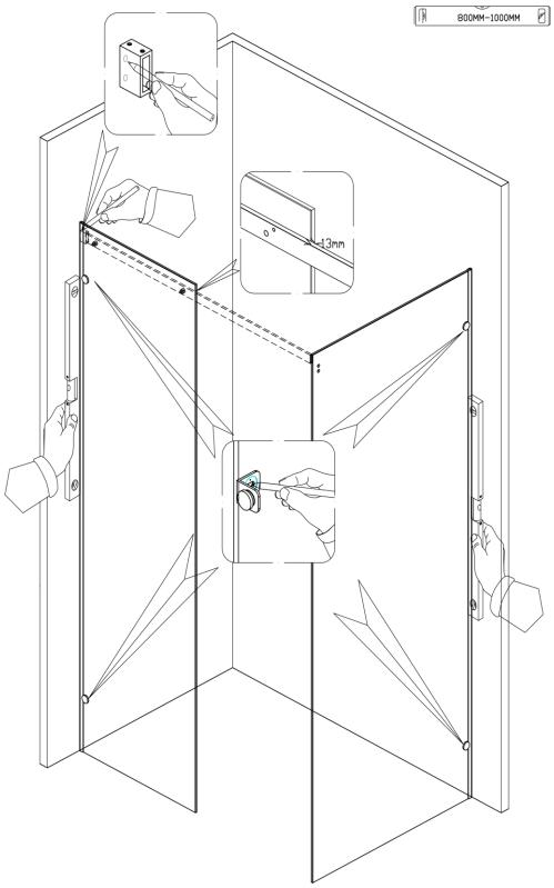
4. Using a spirit level and a pencil, be sure that the side panels will be level before marking where holes will be drilled for the brackets and top rail.
