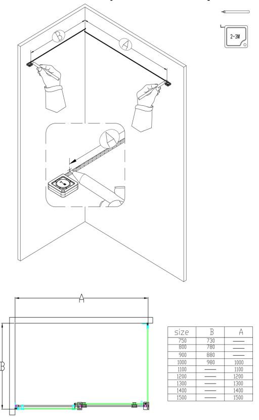
3. Measure and mark where the glass side panels will be positioned.
