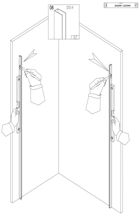
2. Place the aluminium profiles against your walls, using a spirit level and pencil to mark where holes will be drilled.
