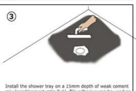
Install the shower tray on a 15mm depth of weak cement mix (sand/cement ratio 5:1). Tile adhesive can be used as an alternate to sand or cement.
